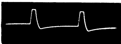
Fig. 19. Unblanking pulse at V7 cathode, 1 \mu sec. recurrent sweep. Amplitude 65 volts.
